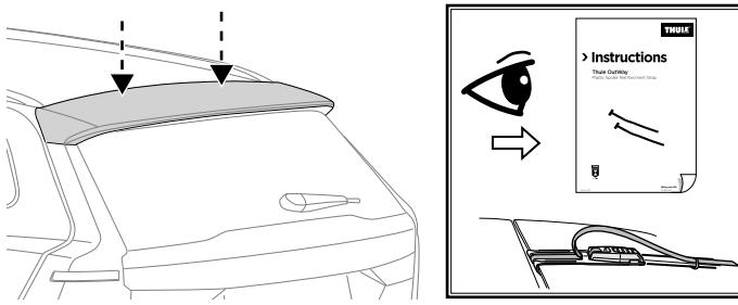
**EN** If plastic spoiler is in the area where upper hooks will be mounted, always use the spoiler kit with the reinforcement strap, according to separate instruction for **Plastic Spoiler Reinforcement Strap**.
